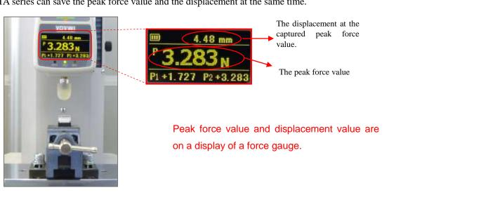
Using function 5 & 6 together realizes easier checking of force-displacement relationships
