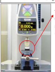
The measurement is started at the setting force applied moment.
